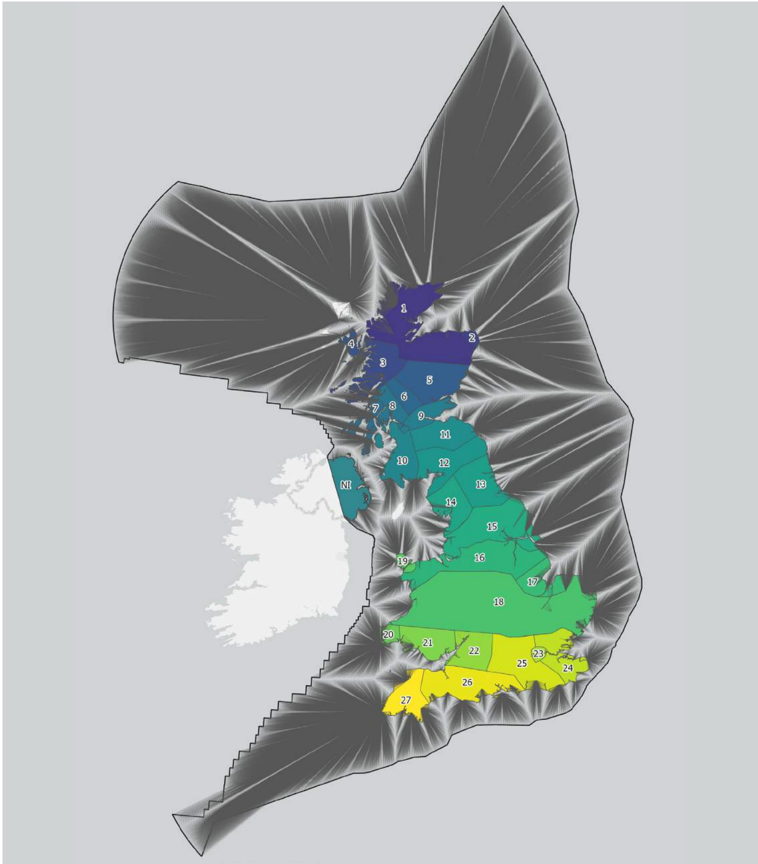
Figure 11. Map showing radial connections of cells to onshore substations. Each cell was assumed to connect radially to the nearest onshore substation in one of the 27 ESO charge zones (plus one additional zone created for Northern Ireland).
