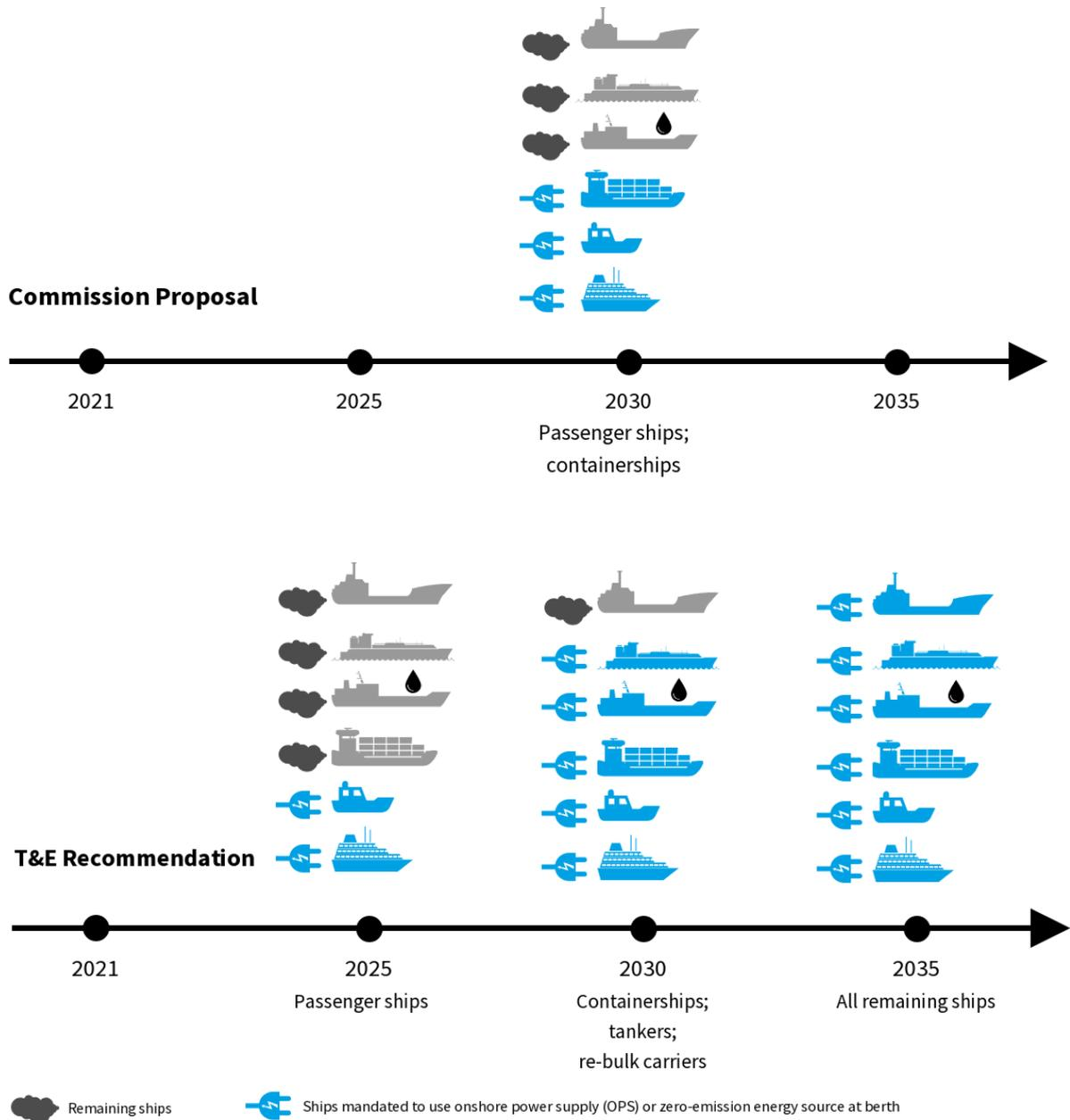
**Figure 14: Commission proposal and T&E recommendation of timelines for the introduction of onshore power supply (OPS) at berth, differentiated by ship type**
