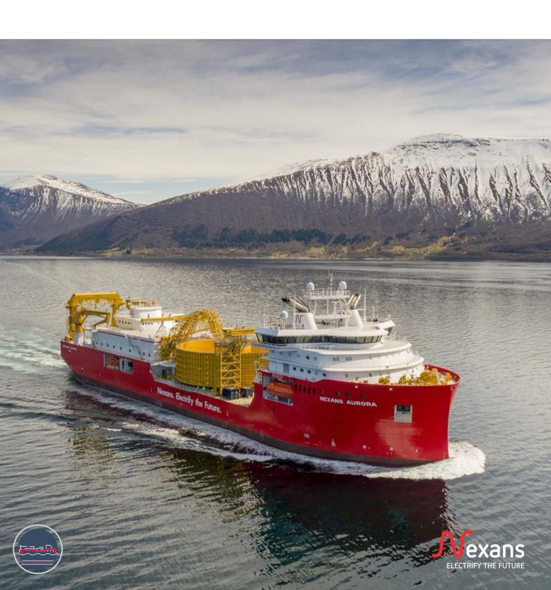
The Vessel is a state of the art and bespoke cable installation vessel for worldwide operations in severe weather conditions, and with high maneuverability and station keeping capacity to ensure a safe and efficient transport and installation of large volumes of HVDC and HVAC cable systems, as well as general subsea construction tasks.
