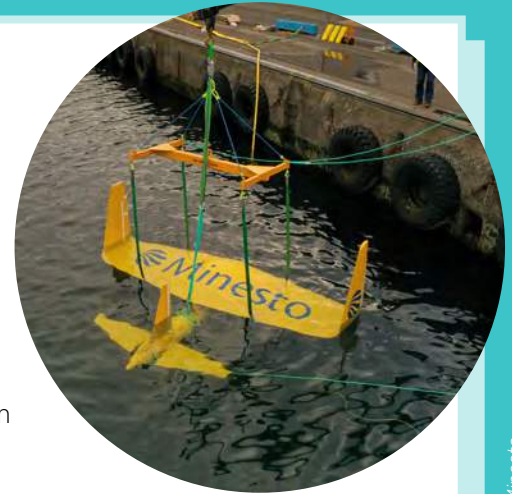
Figure 19: Minesto's tidal kite device
