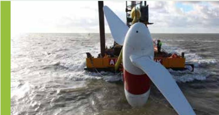
**Tocado Tidal Power** tested its T2 turbine in 2017, as part of the developer's 'Temporary Foundation System'. The demonstration will pave the way for a planned 20 year pre-commercial array, comprised of 5x T2 turbines across their newly developed Universal Foundation Platform System.
