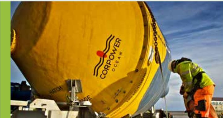
**Corpower** deployed its ½ scale C3 wave energy converter in January 2018. The device has been exposed to real-life sea conditions, following rigorous on-land test program. Testing will allow the demonstration and refinement of low-cost maintenance and inspection operations.
