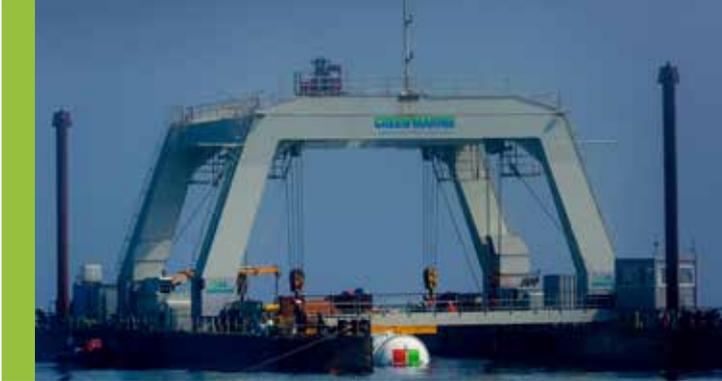
**Naval Energies** installed a Microsoft-owned data centre on the seabed, in June 2018. Powered by ocean energy, sea temperatures will reduce the cooling energy needs by up to 95%. The centre will be immersed for 1 year, but has been designed to operate for 5 years without direct intervention.
