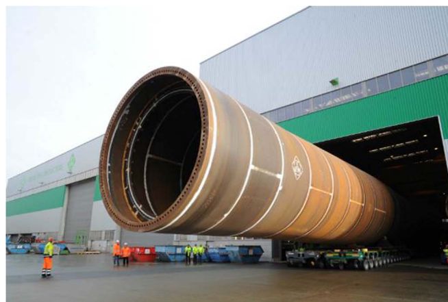
Fig. 4. Monopile of 7.8 m of diameter and 1302.5 t rolled out of the factory in Rostock, used in Veja Mate offshore wind facility ( www.offshorewind.biz/2016/03/14/first-veja-mate-monopiles-reach-eeemshaven/ ).
