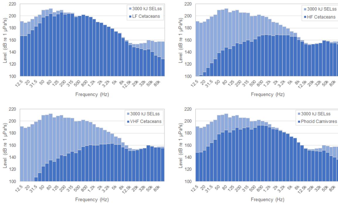
Figure 2-2 Unweighted and Southall et al. (2019) weighted SEL monopile impact piling source level third octave values for LF, HF, VHF and PCW hearing groups for a 3000 kJ hammer
