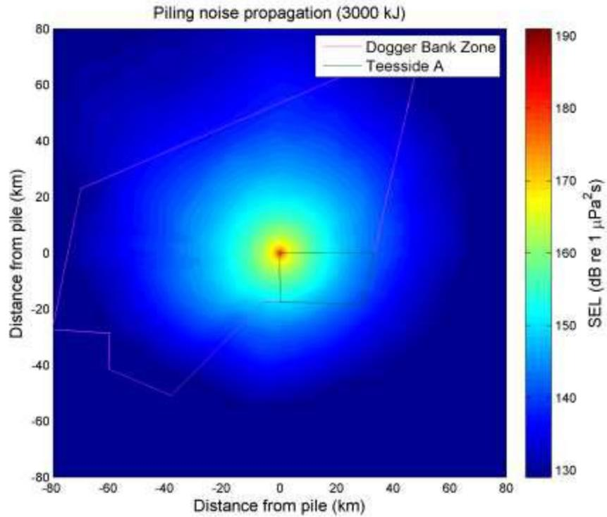
Figure 3-2  $SEL_{ss}$  impact piling noise propagation map for Teesside A location ID1 for a 3000 kJ hammer from the NPL modelling (Figure 4.2 in the NPL report)
