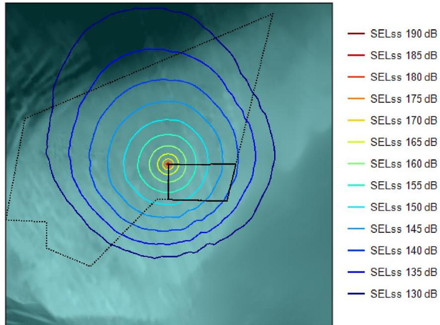
Figure 3-3  $SEL_{ss}$  impact piling noise propagation map for Teesside A location ID1 for a 3000 kJ hammer showing the transmission losses predicted for the INSPIRE modelling, the same colour scale from Figure 3-2 has been used to aid comparison
