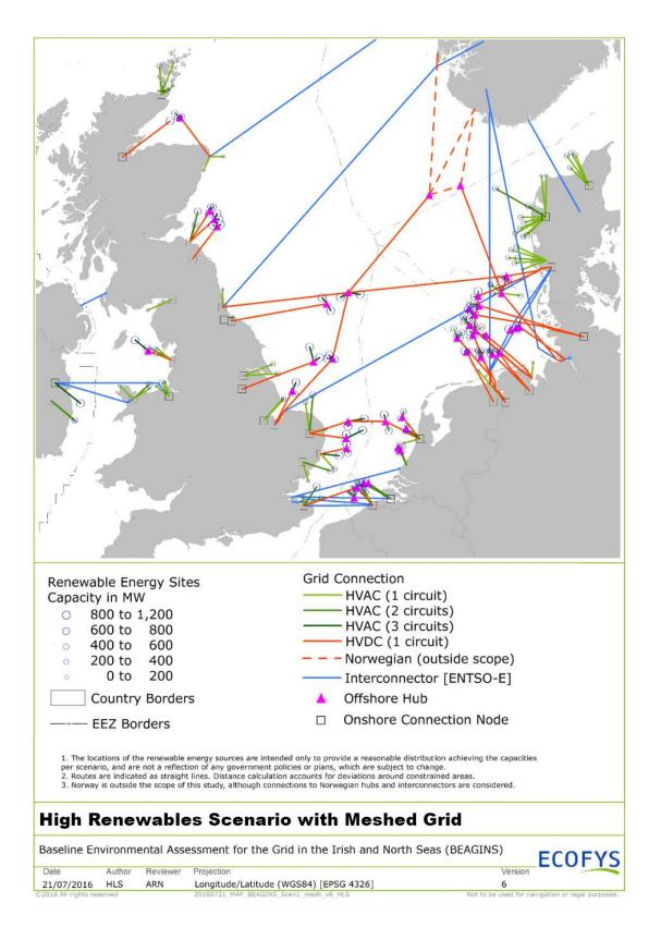
Figure 3-3 - Meshed Configuration to Grid as per High Renewables Scenario
