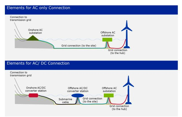
Figure 3-4 - Representation of the Infrastructural Types Considered in an Offshore Energy System
