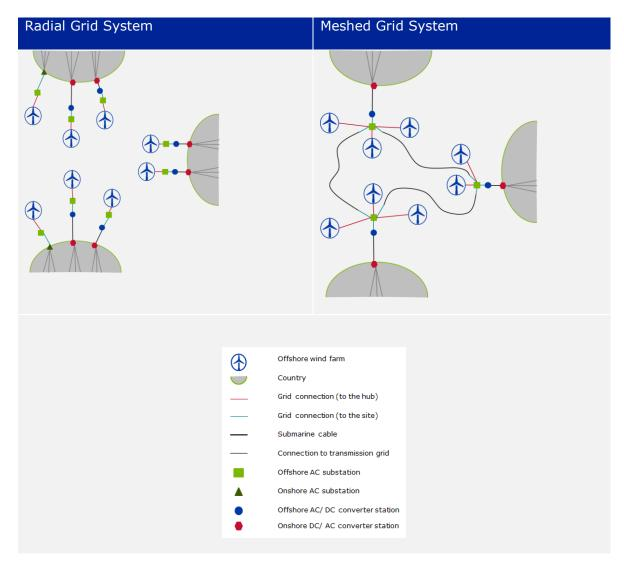
Figure 3-5 - Representation of a Radial and Meshed System
