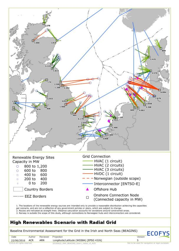
Figure 3-2 - Radial Configuration to Grid as per High Renewables Scenario
